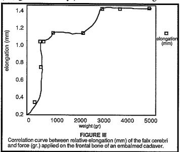
242, 392, 442, 542, 642, 974, 1806, 2850, 3752, and 4654 grams respectively. Each of these weights was applied on the balance trays. A shift between the relative positions of the microphone and the piezoelectric element occurred. This shift produced changes in the observed amplitude of oscillation on the oscilloscope. These changes were recorded by an assistant data recorder. The researcher added equal amounts of weight on each tray each time.
